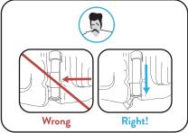
Before placing the Seat, turn the Seat around and make sure the seat belts are slid out to the sides of the tube!
