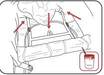
4 Grease your center bolt and mount it in the bottom center loosely so you can align the rest.
