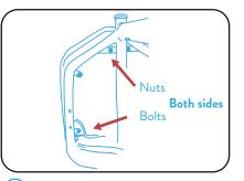
1 Foldable Seat: Loosen 2 nuts and 2 bolts on the back of the Bullitt frame with 5mm Allen Key and 13mm Wrench.
