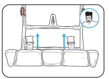
Note! Make sure the seat belt buckles point inwards (underneath the foamy part) before attaching the bolts.
