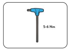
Tighten 2 bolts with 5mm Allen Key.
