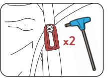
Loosen 2 bolts in the red adjustable mounts with a 5mm Allen Key.
