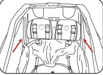
Align Head Rest with the 4 holes (make sure it turns the right way up). Slide the 4 bolts through the holes.
