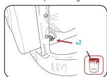
Mount the 2 bolts (from the back /outside of the Canopy) to the tubes (1). Add washers to the 2 bolts. Grease bolts.
