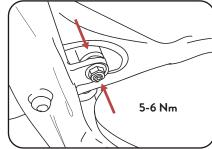
Tighten the nuts, so the Twin Seat tubes sits closely to the frame.
