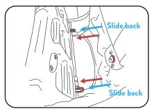
Put center-tube of the Seat in the notch close to the red mounts. Slide the red adjustable mounts back.
