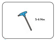
Tighten with 3mm Allen Key.
