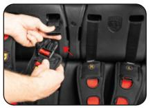
1 The 5-point-Harnesses can easily be converted for use with one child for a more balanced ride.
