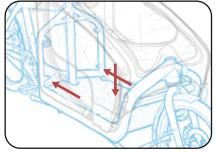
Align bolts with holes in the back (1) and in the center (2) of the Honeycomb Board.
