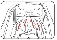
Align 4 holes on the back of the Canopy/armrests with the holes in the Bullitt frame.
