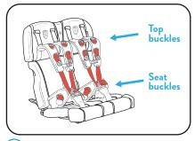
Attach the Harnesses to the buckles! That's 4 buckles for each belt: Two on the Seat, two on the Head Rest.
