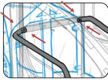
2 Armrest in Canopy: Loosen 2 nuts on the armrest on the inside/outside of the Canopy using 5mm Allen Key and 13mm Wrench.
